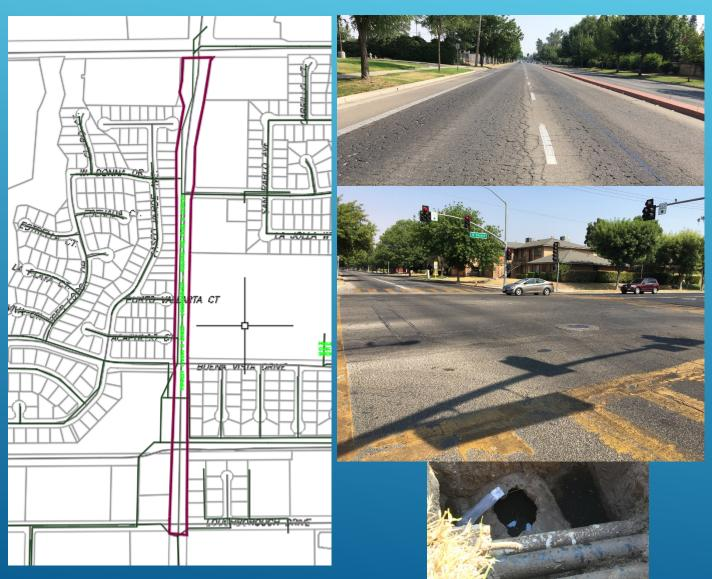
THE CONDITION OF THE ROAD IS SUCH THAT IT CAN NOT BE OVERLAYED AS ORIGINALLY INTENDED. DURING THE SITE VISIT, A WATER LEAK WAS DISCOVERED, UNEVEN ROAD SETTLEMENT IS OCCURING. BETWEEN THE ISSUES AND PCI OF 11 TO 19. FOR THIS REASON A TOTAL RECONSTRUCTION MUST BE DONE
