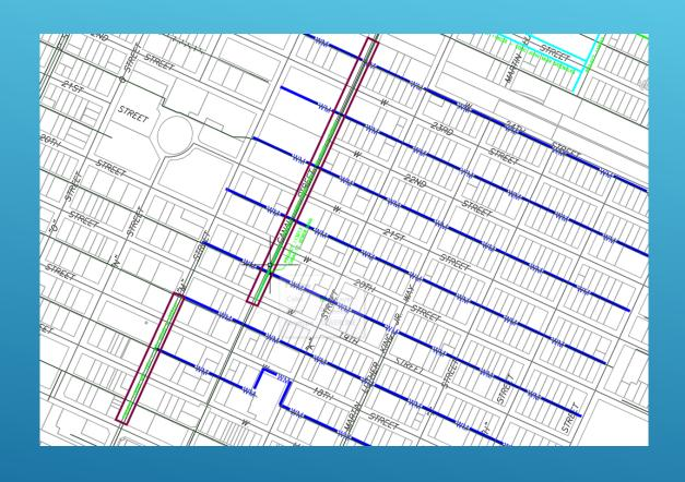
AFTER THE MEASURE V PROJECT WAS INDENTIFIED, IT WAS BROUGHT TO ENGINEERING DEPARTMENT'S ATTENTION THAT THE CITY HAS AGING INFRASTRUCTURE AND NEEDS TO BE REPLACED BECAUSE OF REPEATED WATER BREAK. FOR THIS REASON, THE WATERMAIN NEEDS TO BE REPLACED BEFORE THE ROAD CAN BE REPAIRED
