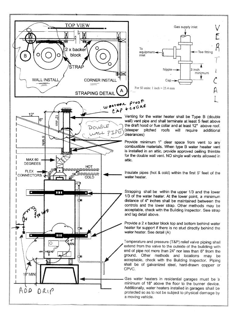
THIS DRAWING DEPICTS MINIMUM CODE REQUIREMENTS PER CRC INFORMATION IS FOR REFERENCE ONLY AND IS NOT A SUBSTITUTE FOR ACCURATE DRAWINGS PREPARED FOR EACH PROPOSED CONSTRUCTION PROJECT.
