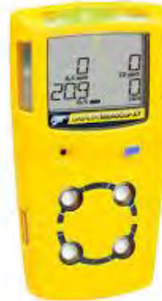
Photo 2-2. Typical Personal Four-Gas Monitor
