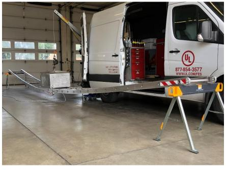
tool that applies 1,000 psi of force to ensure firefighter safety while climbing. A 500 pound load is applied to the middle of each ladder for 5 minutes. The ladder is measured before and after to ensure it does not bend/break. Our 107' TDA and 85' platform aerials received similar testing. Aerial testing included flow tests of the water ways, weighted load test, and a drift test to validate all hydraulic systems.
